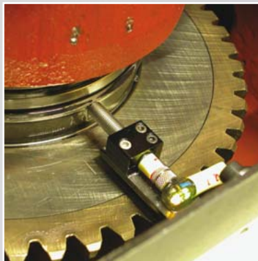
■ Detail of 4 independent overload release clutches
